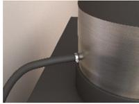
Place a clip over the end of the black high-temperature tube without tightening it.
